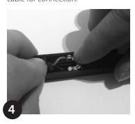
Re-fit terminals, cable and bushings, ensuring all components are seated correctly and within the resin.
