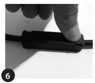
Locate cover and push into place. Leave for a minimum of 5 minutes to dry.
