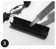
Remove cable, bushes and terminals, and fill 1/3rd to 1/2 of IP67 Slim J-Box with resin (KKJB-07R) between the bushing points.
